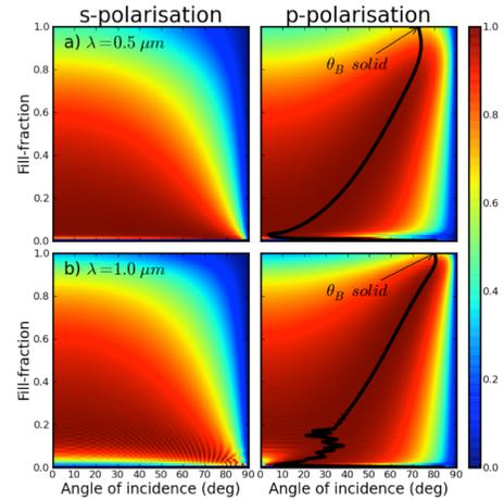
Modelled absorption of very large ( $\sim 20\mu\text{m}$ ) thickness layers  $s$ - and  $p$ -polarization, as a function of fill-fraction and angle of incidence, and for two different wavelengths.
