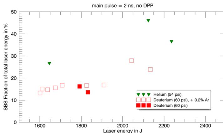
Fig. 1. The backscattered fraction of laser light from SBS is significantly stronger for helium (green triangles) than for deuterium (red squares). Shown here are measurements without the use of a Distributed Phase Plate (DPP).
