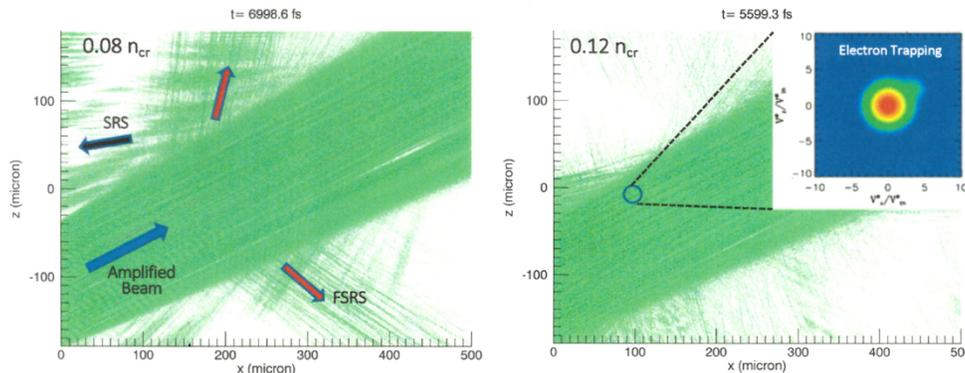
**Figure:** Laser electric field  $E_y$  snapshots of an amplified multi-speckled beam at  $2 \times 10^{14}$  W/cm<sup>2</sup> propagating through a plasma of  $0.08 n_{cr}$  (left) and  $0.12 n_{cr}$  (right). An electron velocity distribution (inset) is sampled at the region circled in black.
